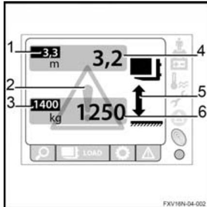
**Example of reading a display with the Dynamic Load Control (DLC) option version 3: weight of the load slightly exceeded**
